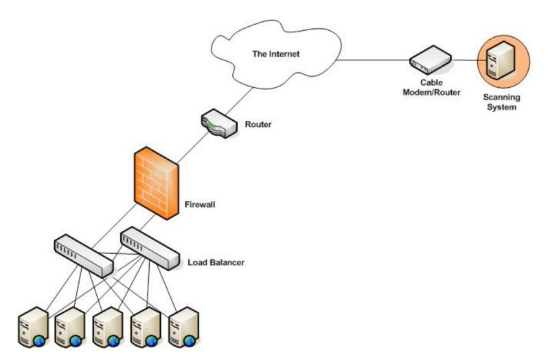
If a remote active operating system fingerprinting tool relies on sending and/or receiving of particular packet types and those packets are dropped by a firewall protecting the target system(s) (or another network obstacle) chances are that the quality of the results would be degraded to the point false results or no results at all will be produced
